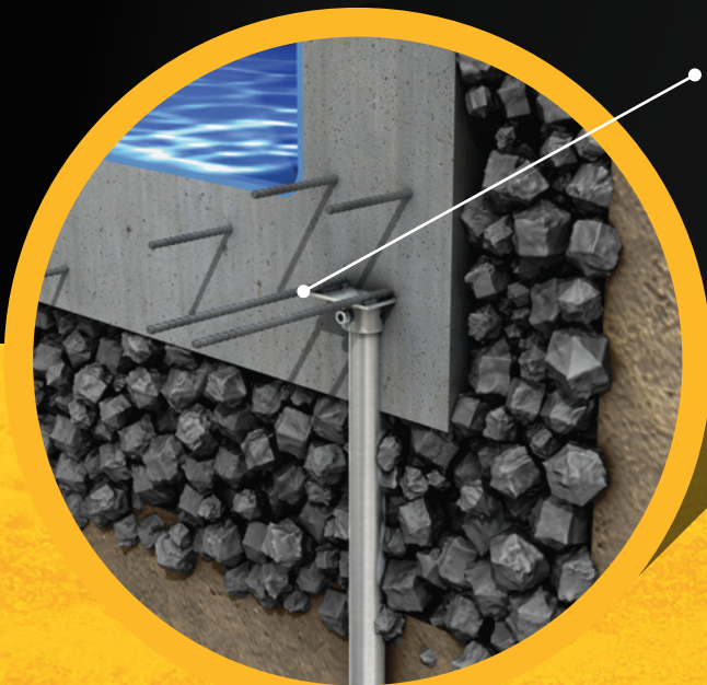
PILE HEAD WITH REBAR
